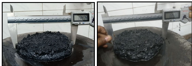
Fig. 5 Free flow of castable E-1, (Left) and T-2, (Right)
