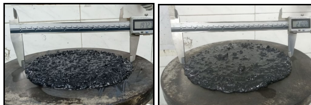
Fig. 6 Tap flow of castable E-1, (Left) and T-2, (Right)
