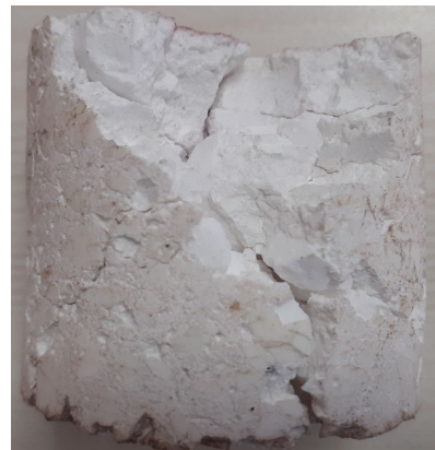
Fig. 8. Disintigration of trial castable after 64 cycles
