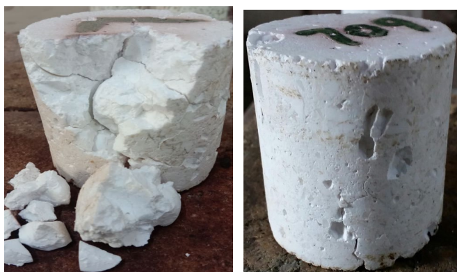
Fig. 7. Appearance of samples after 25 cycles (Left : Regular castable, Right – Trial castable)
