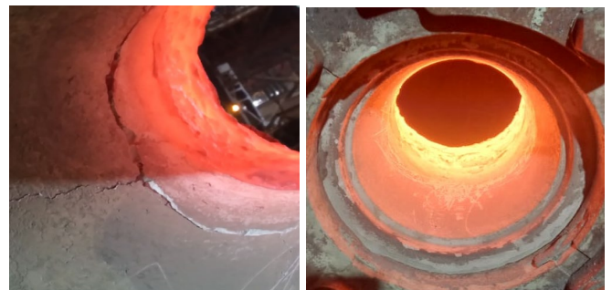
Fig. 13. Appearance of blocks after 48 heats (Left : Regular castable, Right – Trial castable)
