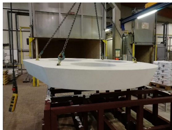
Fig. 5: 4000 kg EAF delta section after drying, liftable at only four anchors
