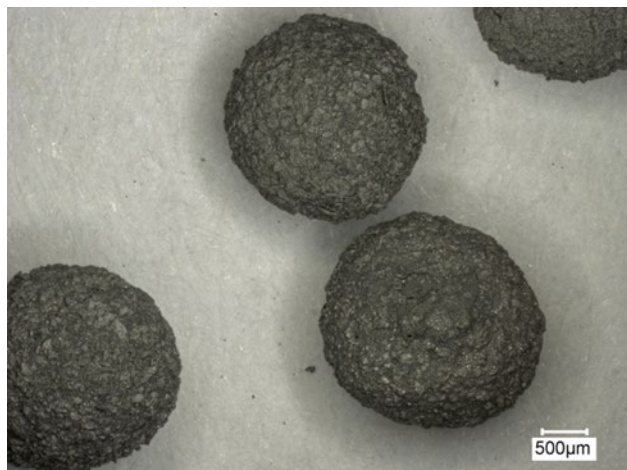
Fig. 5. Photograph of sintered Ta-Al 2 O 3 composite beads with a tantalum content of 60 vol.%.
