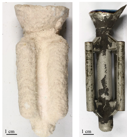
Fig. 3: Images of the shell mould after casting (left) and of the cast part (right).
