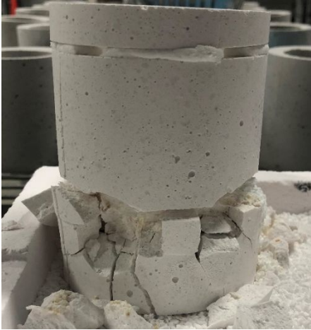
Fig. 2. Post-test 8MAI was unable to be cross sectioned.
