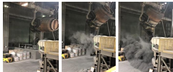
Fig 1. Scattered dust in the tilting process
